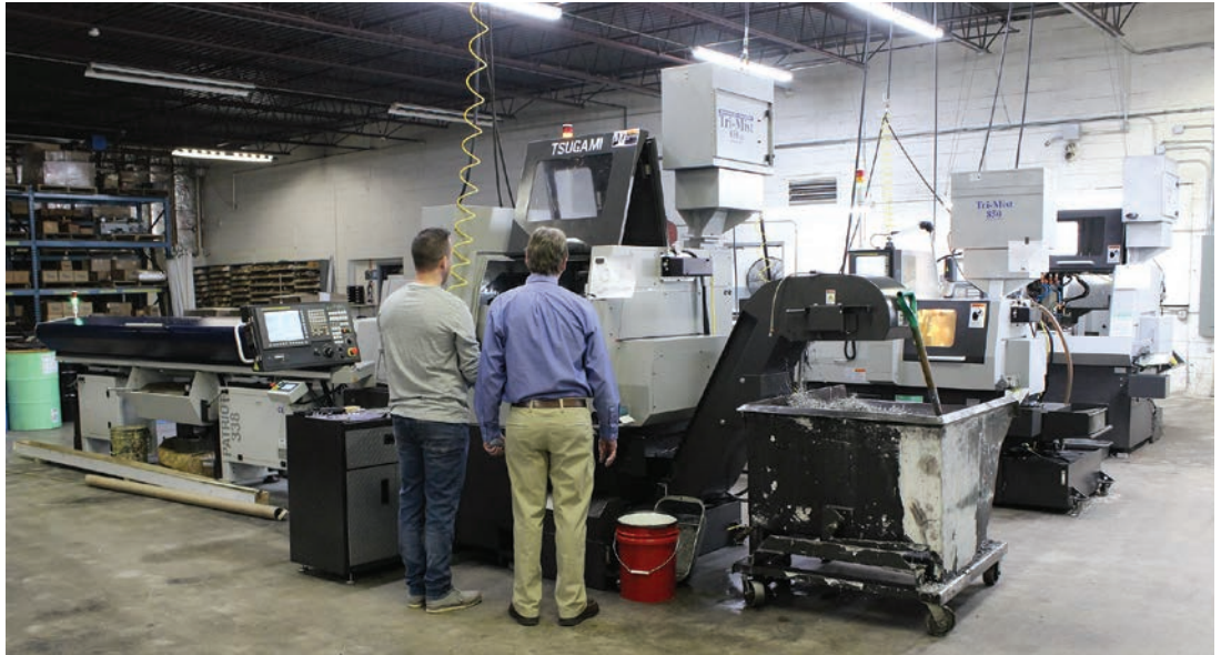
Operators at Radax Industries program the Tsugami. The machine is fitted with an Edge Technologies Patriot 338 bar feeder to increase productivity.
