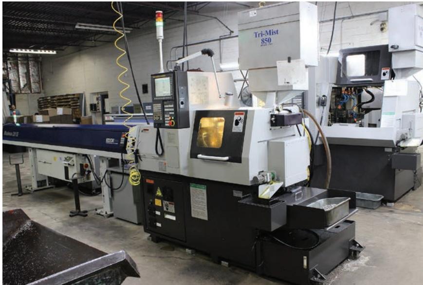
The Tsugami is equipped with an Edge Technologies Minuteman 320 SE bar feeder and a Tri-Mist 850 coolant filter. A parts catcher moves components to the outside of the machine to facilitate lights out machining.
